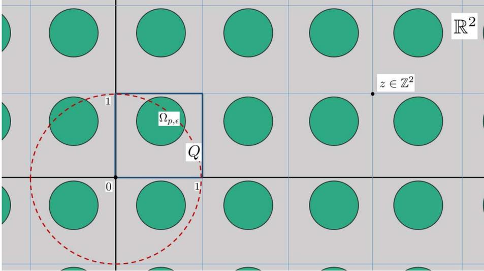
Figure 2.1: The composite with the inclusions in the form of a disk
