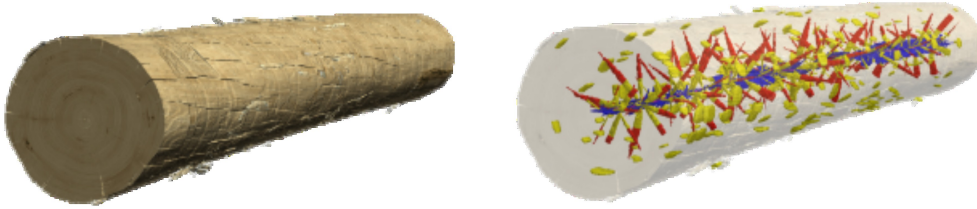
Figure 2.9: 3D volume from CT data (left) and extracted log model (right)
