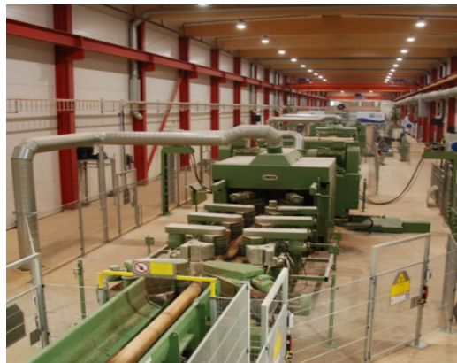
Figure 2.3: A typical high speed log cutting line
