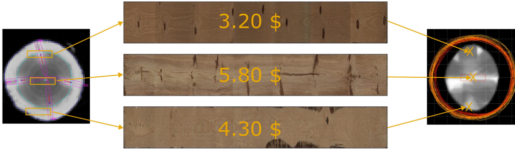
Figure 4.4: Example of a V-Map. On the left, a tomographic section of the measured log with defects highlighted and three possible placements of a board. In the middle, the surface of the board obtained from each of these three placements, where the corresponding value is shown. On the right, the value map related to this board, where the value of the three points shown corresponds to the value of the boards (black points identify value 0, white points the maximum value).
