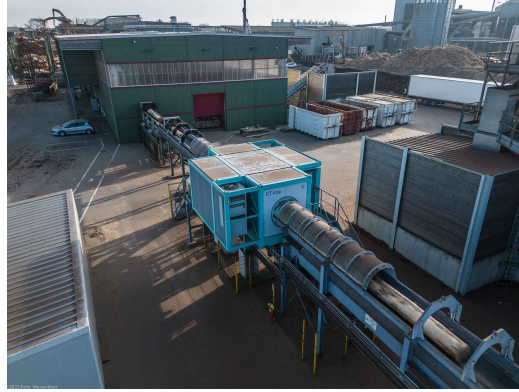
Figure 2.5: A CT scanner installed in a sawmill
