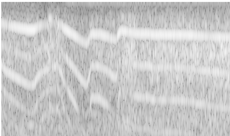
Figure 5.1: Spectrogram of an accelerating car engine. The fundamental and two of its harmonics can be easily recognized.
